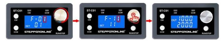
In the menu setting interface, Turn the knob to change the parameter codes F-01~F-13. Long press the knob, save the parameter and exit, enter the running interface.
