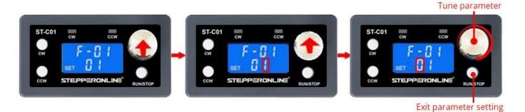
In the menu setting interface, **short press** the knob to enter the F-XX, Corresponding menu parameter setting status. **Short press again** to shift, rotate the knob to adjust the parameters. **Short press the RUN/STOP button** to exit the parameter setting and return to the main menu number adjustment interface.
